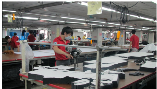
Fig. 4b. Fabric cutting operation.
