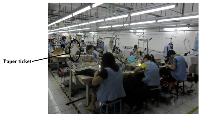
Fig. 3. Using paper tickets to record progress in production operations.
