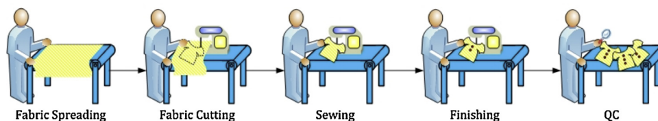
Fig. 5. Production operation flow in the garment industry.
