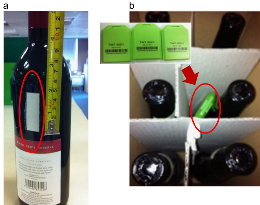
Fig. 5. (a) RFID tag and (b) battery-assisted cold chain tag adopted in the case study.
