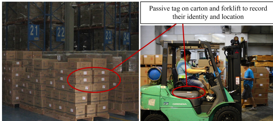
Fig. 5. Passive RFID tags on cartons and forklift.
