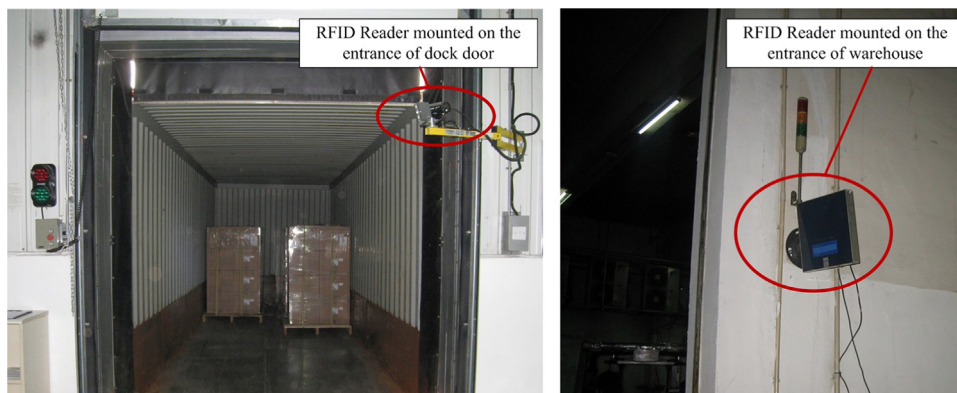
Fig. 6. Passive RFID reader on the dock door and on the entrance of the warehouse.
